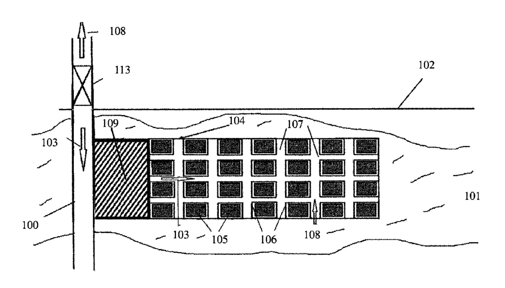
production and injection are proposed. Methods for fluids production, injection and recovery using hydraulic fracturing method are proposed. The proposed method increase the well lifetime due to reduced fluid flow impact on fracture walls and proppant clusters.
