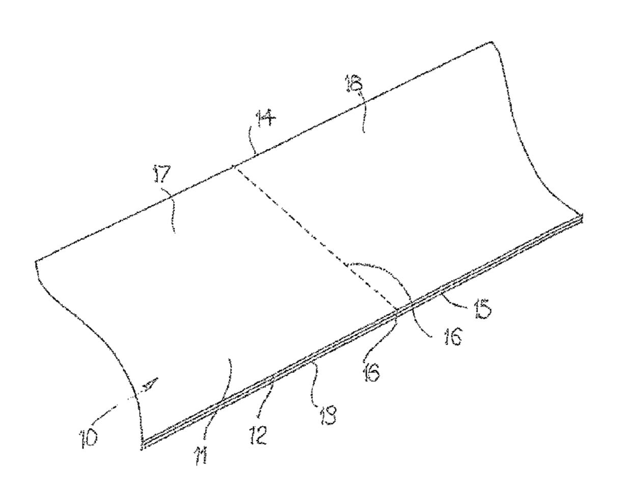
in use, an outwardly facing adhesive surface, and a second adhesive substrate extending substantially across the width of said wrapping material and being adhesively secured to said first surface of the wrapping material whereby the second adhesive substrate overlies said line of perforations.
