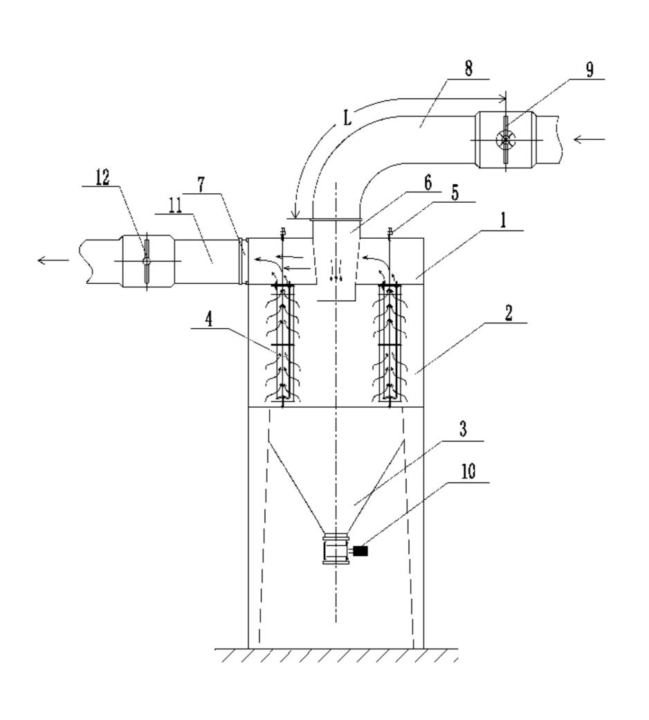
time  $\Delta T$ , the valve on the exhaust gas inlet pipe and/or the purified gas outlet pipe is opened to continuously perform the dedusting. The present invention provides a new dedusting mode with the "super accumulation shelf layer," which significantly improves the filtration accuracy and the dedusting efficiency of the dust remover.
