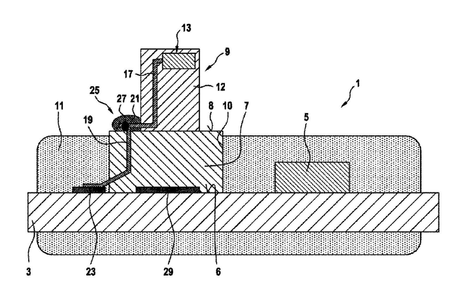
protective compound. Connection elements of the socket element and connections of the second component are connected via a welding connection. Second components are attachable to the circuit board in a reliable manner.
