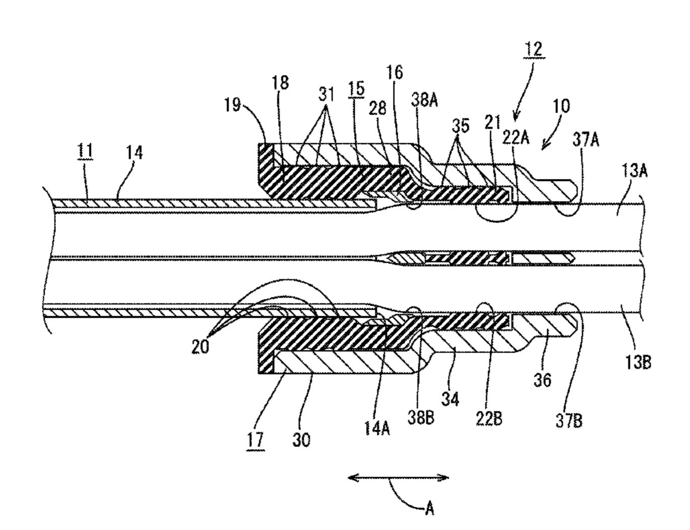
respectively. The guide member is located more to a rear than the electric wire through portion in an extending direction in which the first to the fourth electric wires passed through the first to the fourth through holes extend. The guide member includes first to fourth guide holes through which the first to the fourth electric wires are passed and aligned with the first to the fourth through holes.
