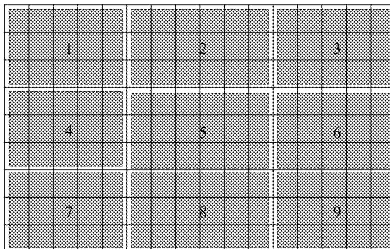
gained subarea backlight value is below a first threshold, then the corresponding backlight value adjustment coefficient is less than 1; and a subarea backlight value outputting section configured to output the respective adjusted subarea backlight values to driver circuits of backlight sources in the corresponding backlight subareas to control the brightness of the backlight sources in the corresponding backlight subareas as a result of driving.
