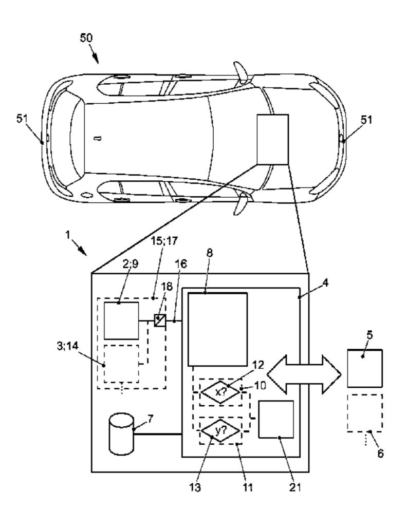
of the vehicle so that a predefined trajectory is travelled autonomously, wherein the controller has an obstacle-detection device to detect obstacles in the surroundings of the vehicle, wherein the at least one sensor system has at least one acceleration sensor, and the obstacle-detection device uses measurement data collected by the at least one acceleration sensor to detect collisions with obstacles.
