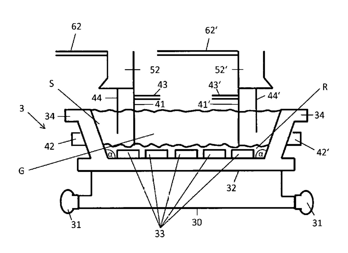
first layer is applied as a hearth layer on a grate surface of the pallet car. In at least one second step a second layer at the same time or successively is applied as a side layer on two opposed side walls of the pallet car and a third layer is applied as green pellet layer between the side layers and on the hearth layer. The pellets used for the grate and the side layer differ in terms of their diameter and size distribution.
