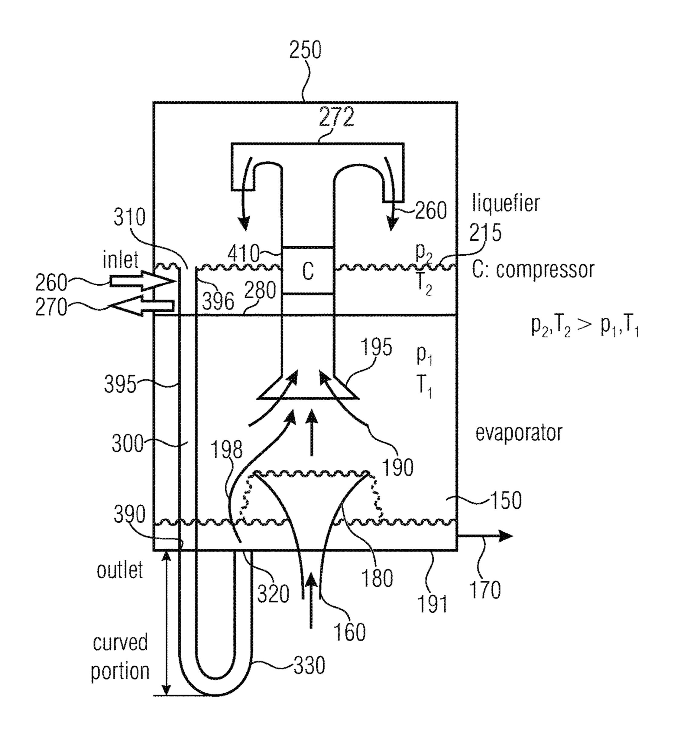
heat pump operation:  $\Delta T = T_2 - T_1$
