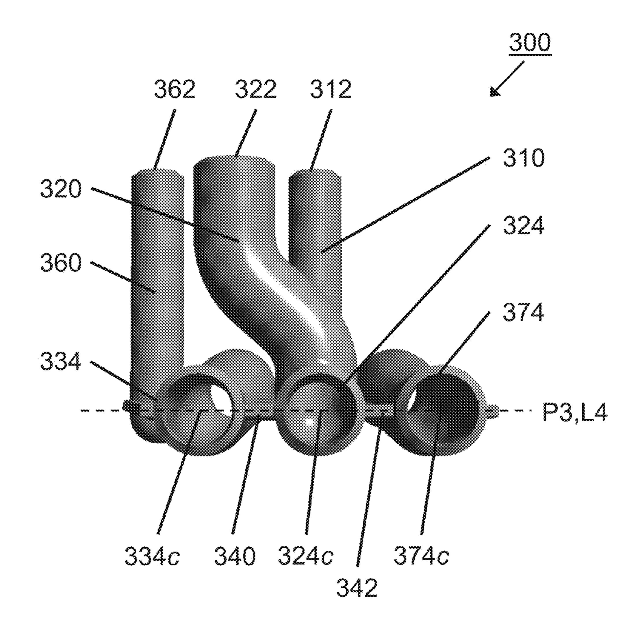
Fig. 16 (bottom view of lower transition casting)
