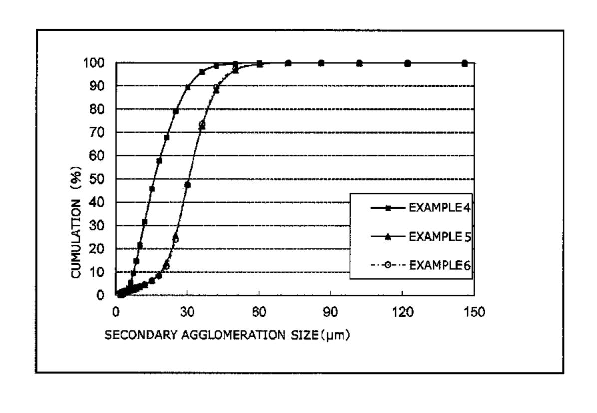
(D<sub>90</sub>-D<sub>10</sub>)/D<sub>50</sub> is less than 6. The decontaminator is made by adding a ferrocyanide aqueous solution and an aqueous solution containing at least one transition metal into a suspension liquid containing a precursor formed by magnetic particles coated with organic monomer or polymer while applying a strong shear force.
