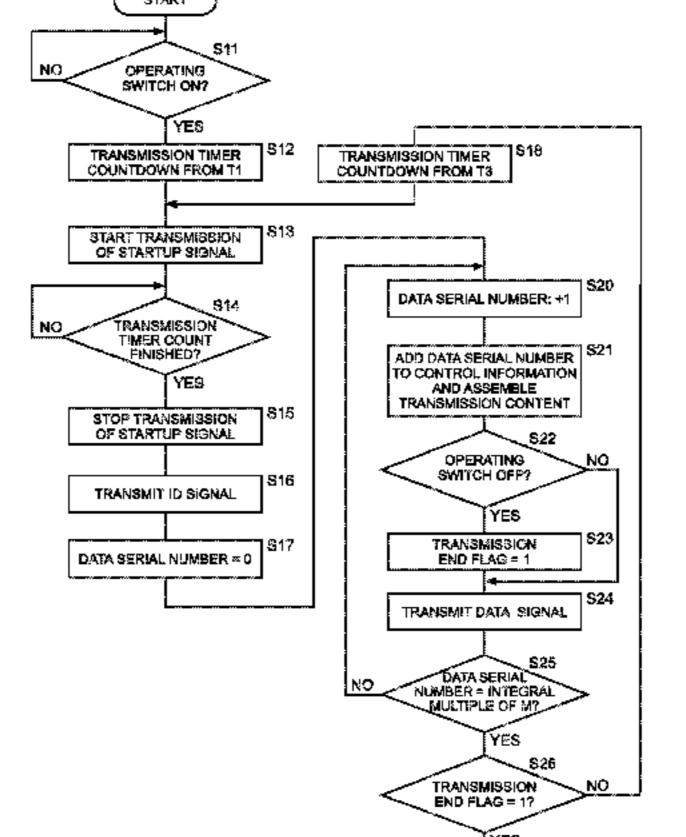
signal, the portable machine adds the ID signal into the wireless signal each time M data signals have been transmitted, and continues to transmit the wireless signal. Meanwhile, each time the vehicle-mounted machine receives the ID signal included in the wireless signal, the vehicle-mounted machine verifies the identification information the received ID signal against identification information stored in a ROM, and continues to receive the wireless signal when there is a match.
