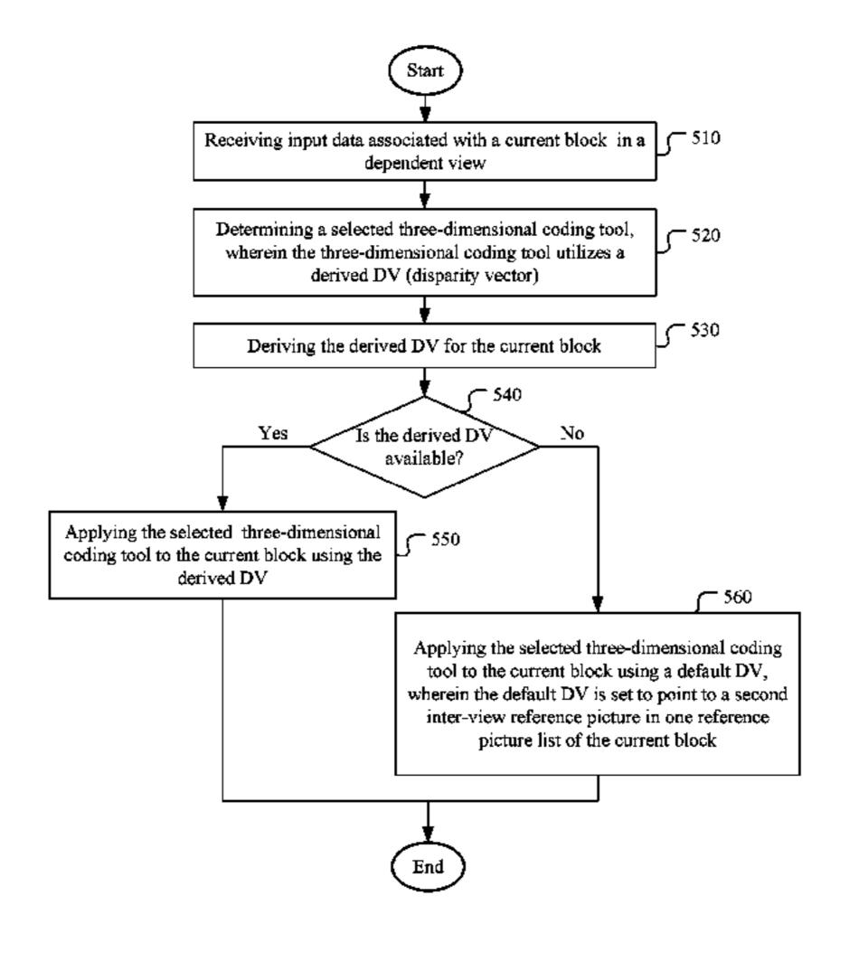
default DV is set to point to an inter-view reference picture in a reference picture list of the current block.
