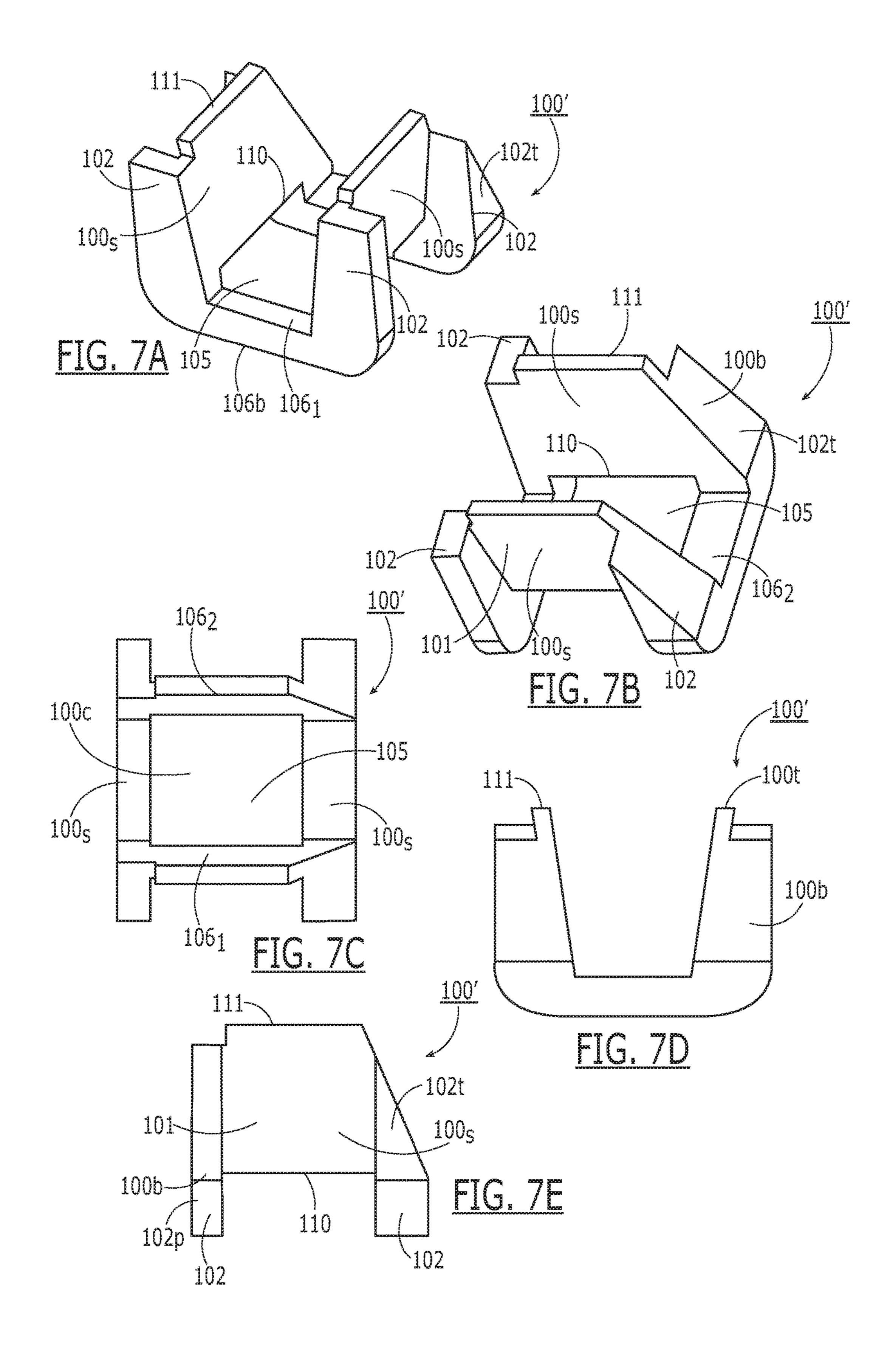
The floor of the metal arc chute resides on an internal planar wall of the molded circuit breaker case.
