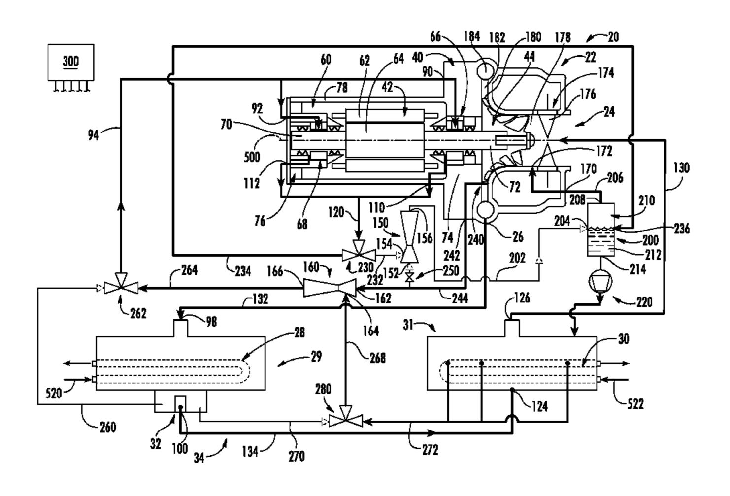
202, 206) are coupled to the bearings to pass fluid along a drain flowpath from the bearings to a location (172) upstream of the impeller and downstream of the IGV array.
