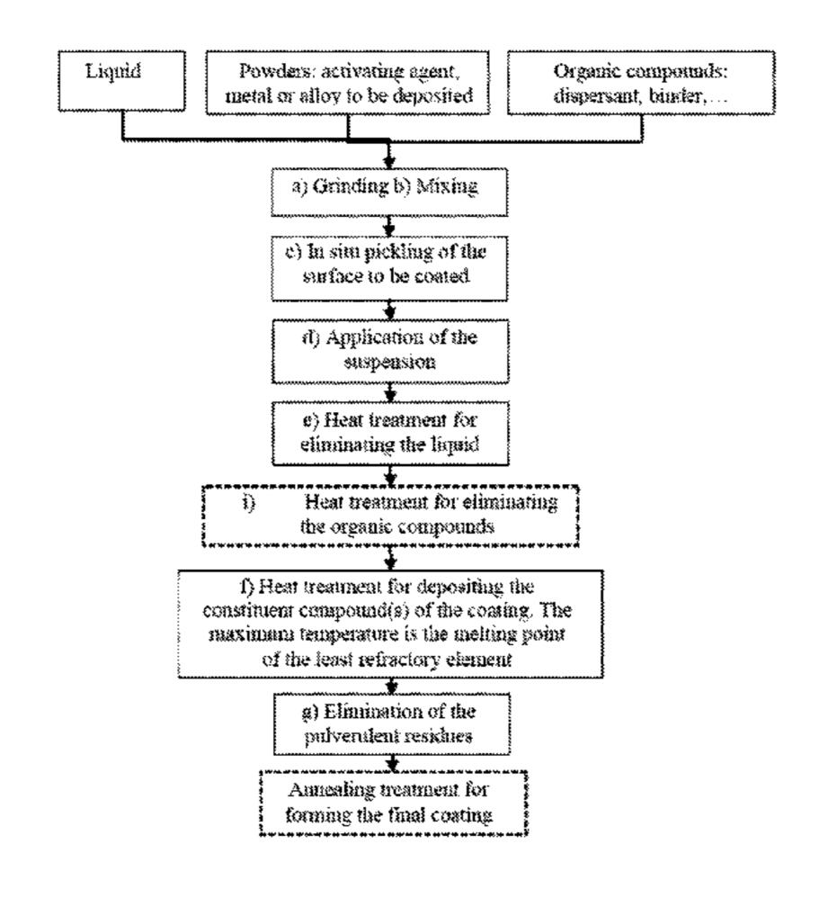
ders of an activating agent and a powder of the metal or of the alloy to be deposited on the substrate that were ground in step a) and a liquid so as to form a suspension, and a step of applying the suspension to the portion of the substrate to be coated.
