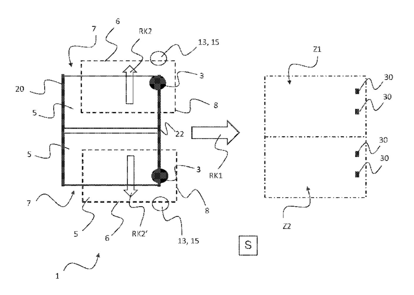
ing, preferably by means of optical detection, an outer edge (6) of the particular intermediate layer (5). Subsequently, the removed individual intermediate layers (5) move toward a particular target location (Z1, Z2), the particular, preferably optical detection thereby being taken into account, such that the intermediate layers (5) reach their particular target location (Z1, Z2) in a predetermined position.
