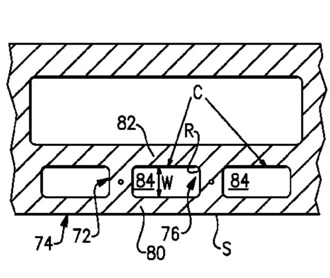
which an amount of internal residual stress in the single crystal microstructure exceeds the critical internal residual stress. The internal cavity includes a cross section less than about 20 mils near the corner radius.
