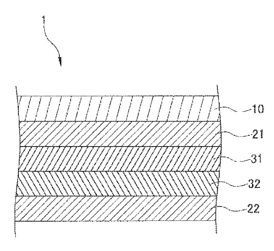
overlapped, is between 0.20 and 0.45. The filter medium can be used in a filter pack or filter unit, and may be produced by integrating the first and second films and the pre-collection member using heat lamination.
