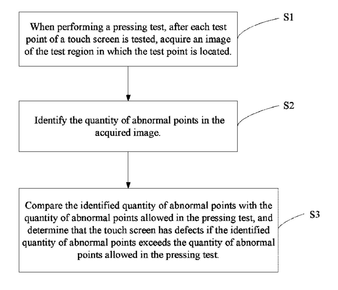
can check instantly and accurately whether defects arise on the touch screen during the pressing test.
