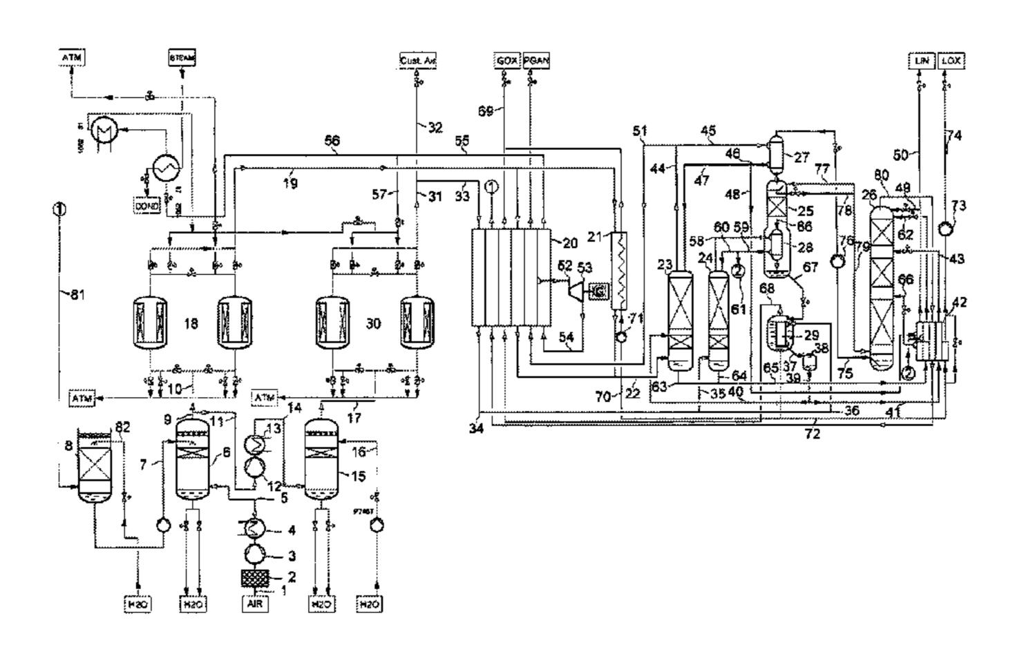
higher than the first total air pressure. The re-compressed second partial air stream (14) is cooled with cooling water in a second direct contact cooler (15) by way of direct heat exchange (13, 15). The cooled second partial air stream (17) is purified under the higher pressure in a second purification device (30), thus generating the second purified partial air stream (31).
