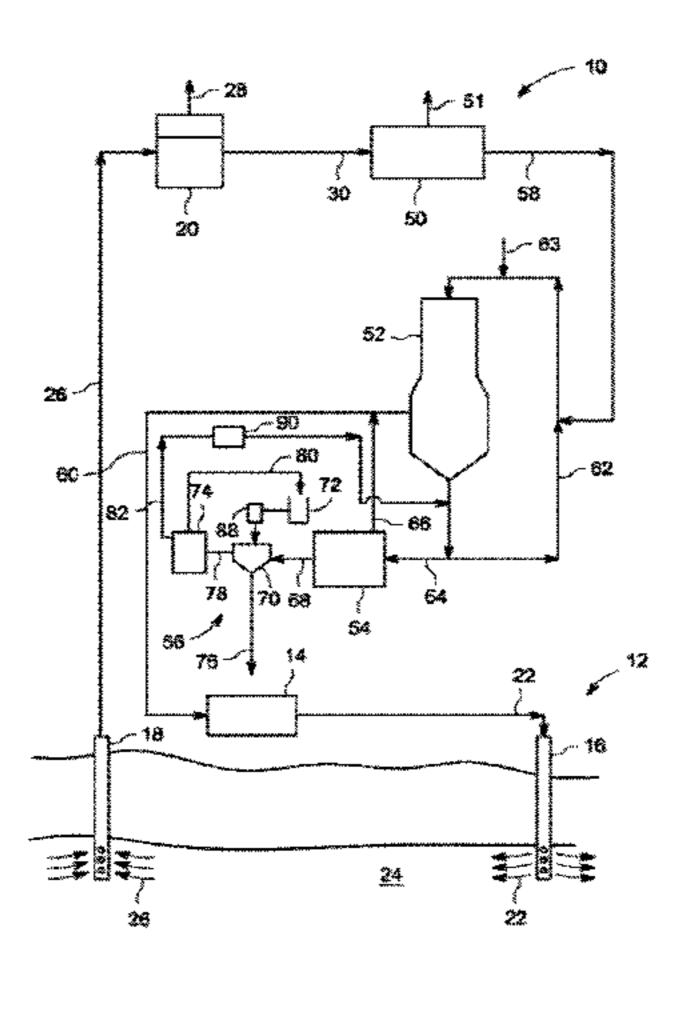
added to the blowdown or slurry. The solids precipitate and are separated from the blowdown or slurry. The solvent may be recovered for re-use in treating more blowdown or slurry.
