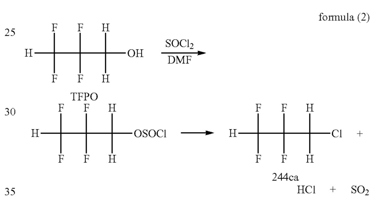
In a reaction of the formula (2), as a reactor, a commonly-used reactor, such as a glass flask, an autoclave made of SUS, and a glass-lined reactor, can be used. When the glass flask is used, it is preferable to place a glass distillation column packed with a Raschig ring and simultaneously perform production and separation of 244ca.
