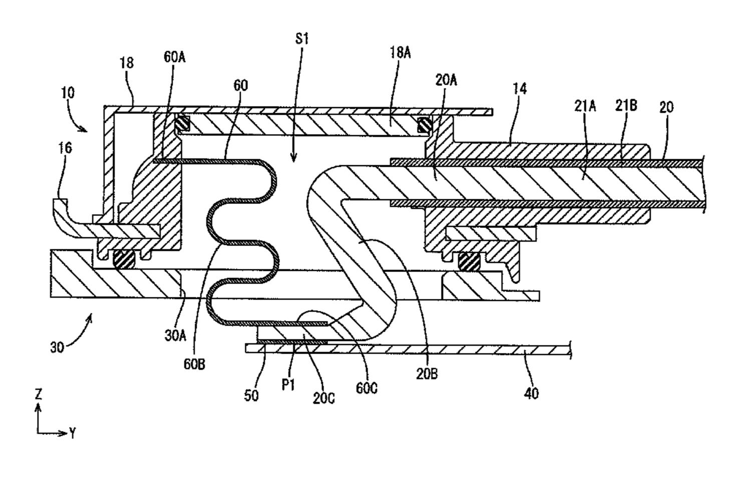
held in the body portion (14) and extending from the body portion (14) toward the connecting portion (20C). The spring member (60) includes a contact portion (60C) configured to give a spring property to the connecting portion (20C) by being held in contact with the connecting portion (20C).
