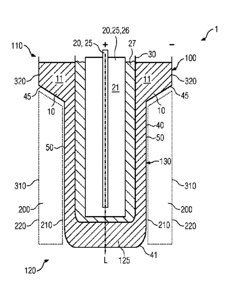
heat from the electrochemical storage device via a first surface and/or to supply heat thereto and to supply and/or receive heat via a second surface. A receiving section is in thermal contact with the heat dissipating device.
