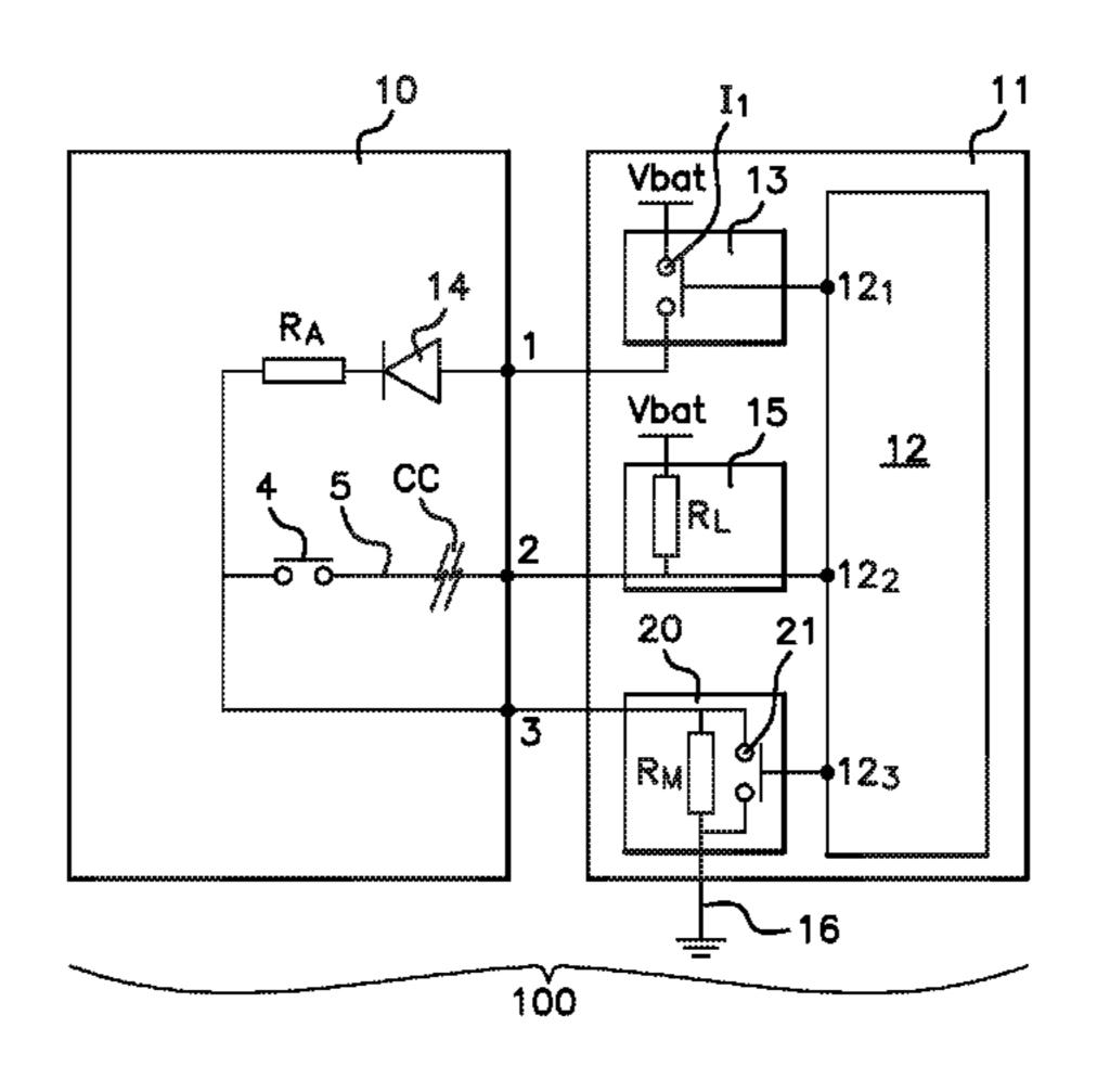
comparing the two read values in order to diagnose a short-circuit to ground fault of the start/stop unit.
