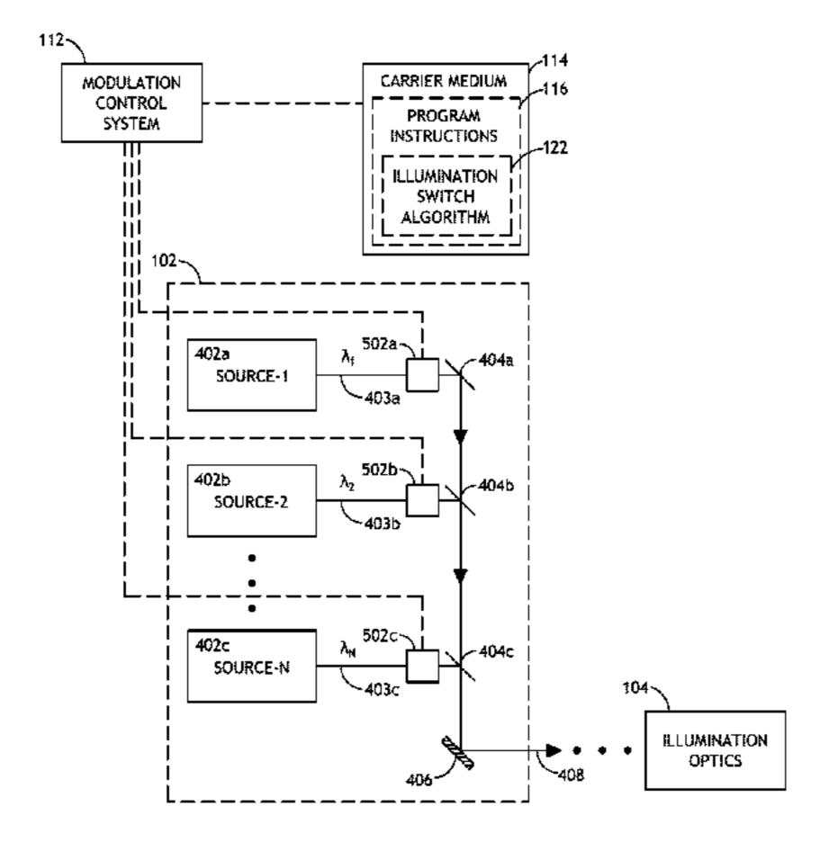
length. In addition, the present invention includes the time-sequential interleaving of outputs of multiple light sources to generate periodic pulse trains for use in multi-wavelength time-sequential optical metrology.
