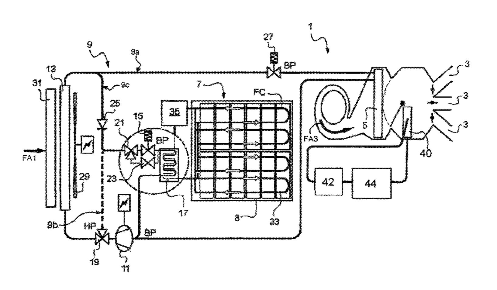
controlling the temperature of an automobile battery (7) implemented by means of such heating, ventilation and/or air-conditioning equipment (1).
