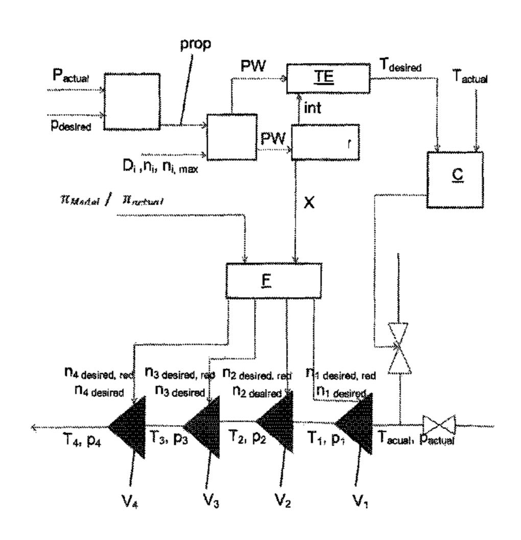
inlet temperature and the actual speed for each compressor is adjusted to the determined desired speed.
