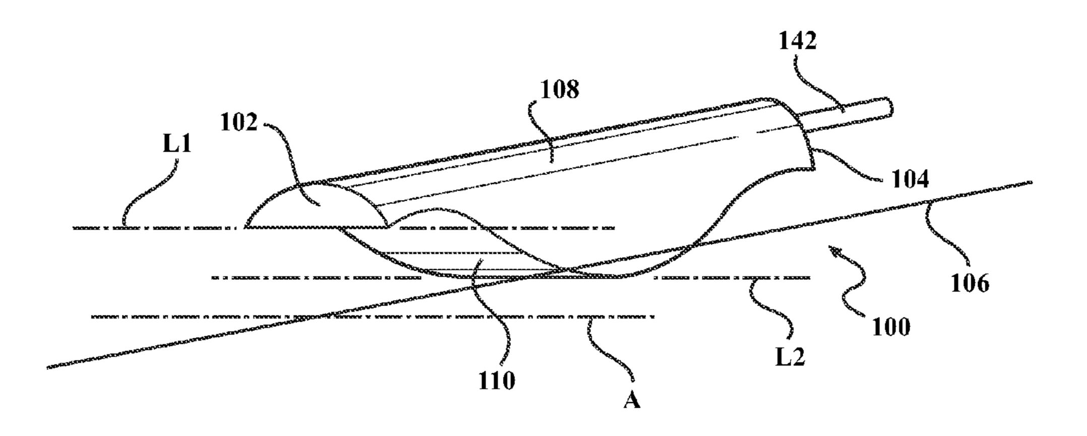
to move the valve (100) relative to the exhaust passage (18) so as to control exhaust gas pressure within the exhaust passage (18). In some embodiments, a pilot tube (280) is used in combination with the valve (100) to generate high pressure exhaust gas recirculation at the engine (12) intake.
