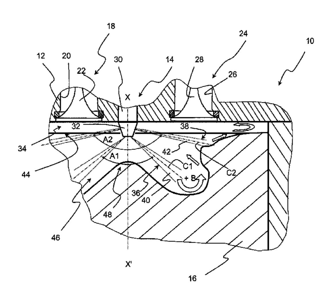
injected so that an axis C1 of the lower sheet jets is contained between center B and projection (48).
