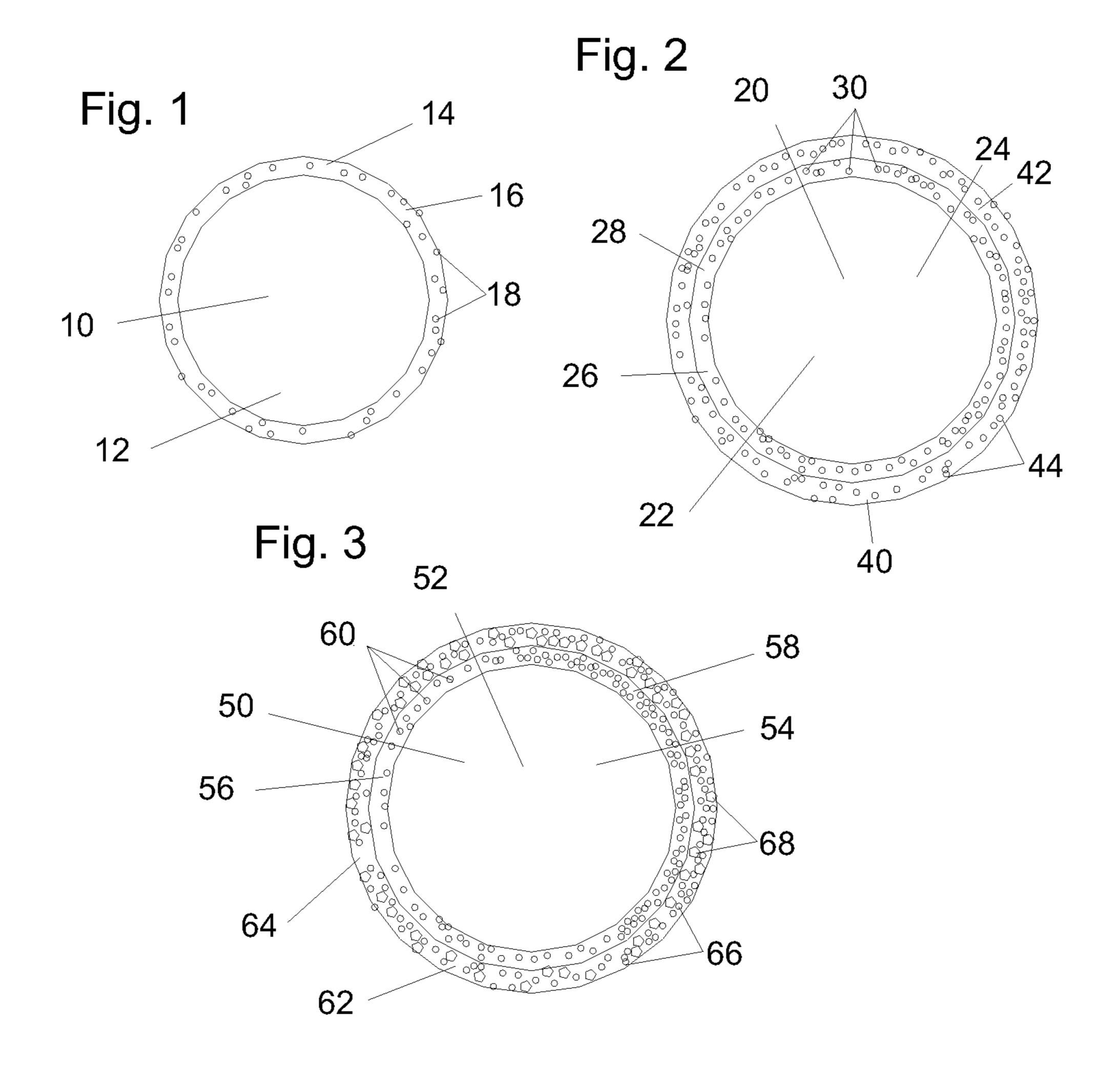
COATING COMPOSITIONS FOR ROOFING GRANULES, DARK COLORED ROOFING GRANULES WITH INCREASED SOLAR HEAT REFLECTANCE, SOLAR HEAT-REFLECTIVE SHINGLES AND PROCESS FOR PRODUCING THE SAME
