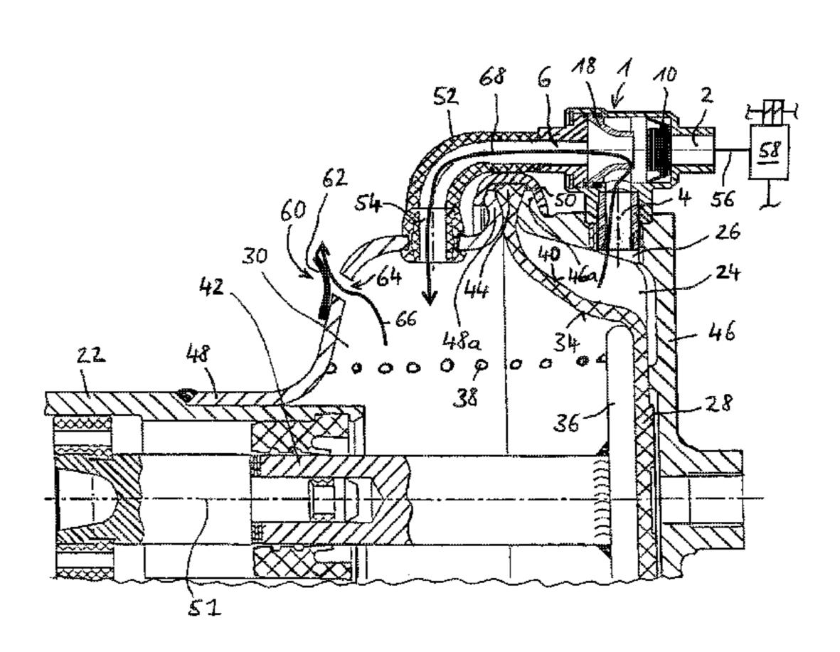
between the brake line and the pressure chamber is arranged to connect the brake line to the pressure chamber when the pressure in the brake chamber is greater than in the pressure chamber, and to connect the pressure chamber to the spring chamber when the pressure in the pressure chamber is greater than the brake line pressure.
