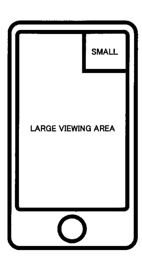
assigned thereto, and a display control unit which displays the image in the first viewing area and the image in a second viewing area other than the first viewing area among the plurality of viewing areas concurrently based on a result of the discrimination by the operation determination unit.
