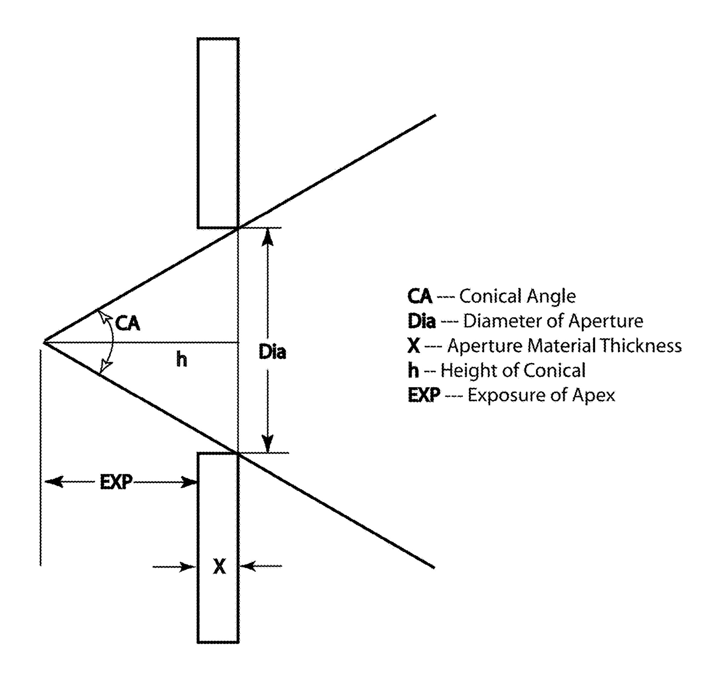
The Exposure (EXP) of the Apex = Height of Conical (h) - Aperture Thickness (X)
