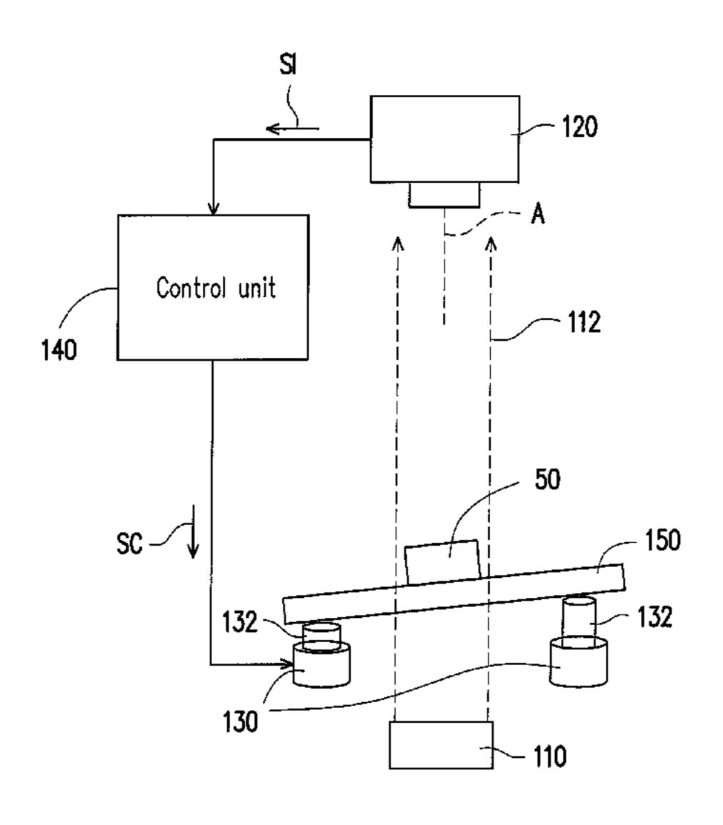
configured to pick up images of the object respectively corresponding to the at least three values. The control unit is configured to calculate the relative angle between the object and the image pickup device.
