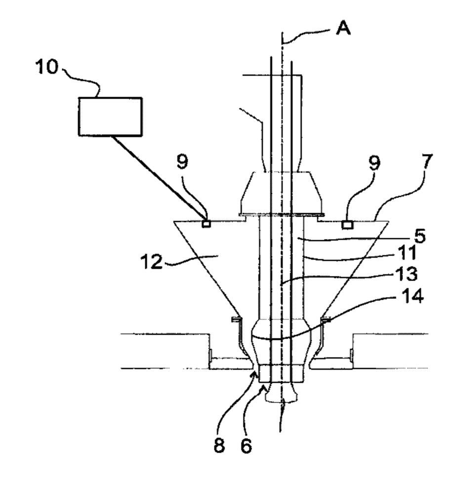
up into the reaction shaft. The arrangement comprises at least one imaging means for producing images representing the cross-section of the reaction gas channel, and a processing means for receiving images of the cross-section of the reaction gas channel from the imaging means.
