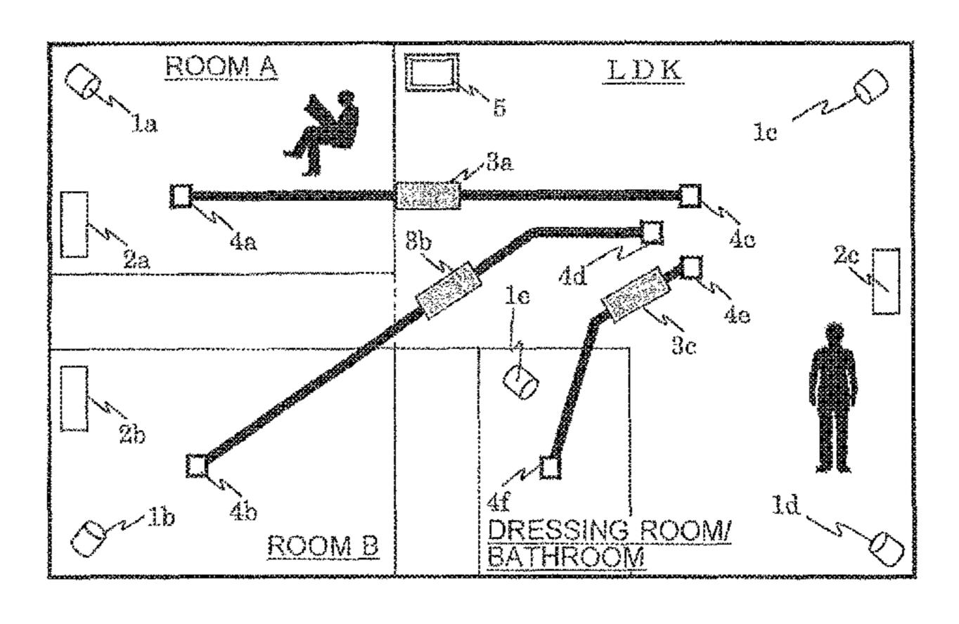
senting a number of humans present per unit time in each of the plurality of rooms, on a basis of a past result of detection by the human detector, and a controller configured to control the air circulation device and the air-conditioning apparatus on a basis of a result of estimation by the optimal airconditioning ventilation operation estimating unit.
