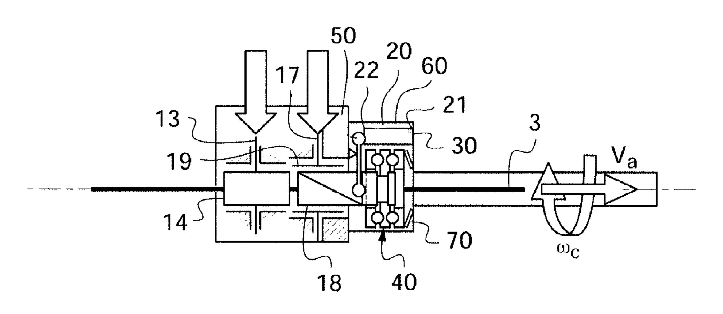
order to cause it to oscillate translationally so as to superpose an axial oscillation component with the feed movement.
