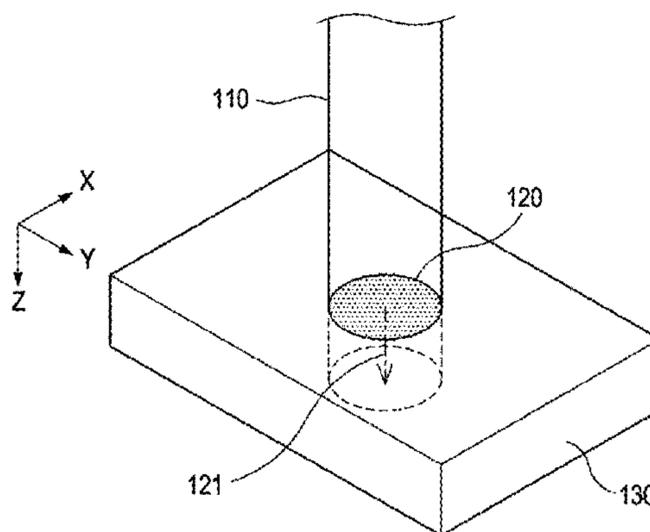
measured are acquired, so as to measure a depth direction movement of the object to be measured, and can correct the phases of interference signals on the basis of the measured depth direction movement, so as to generate an OCT image which is compensated for the depth direction movement.
