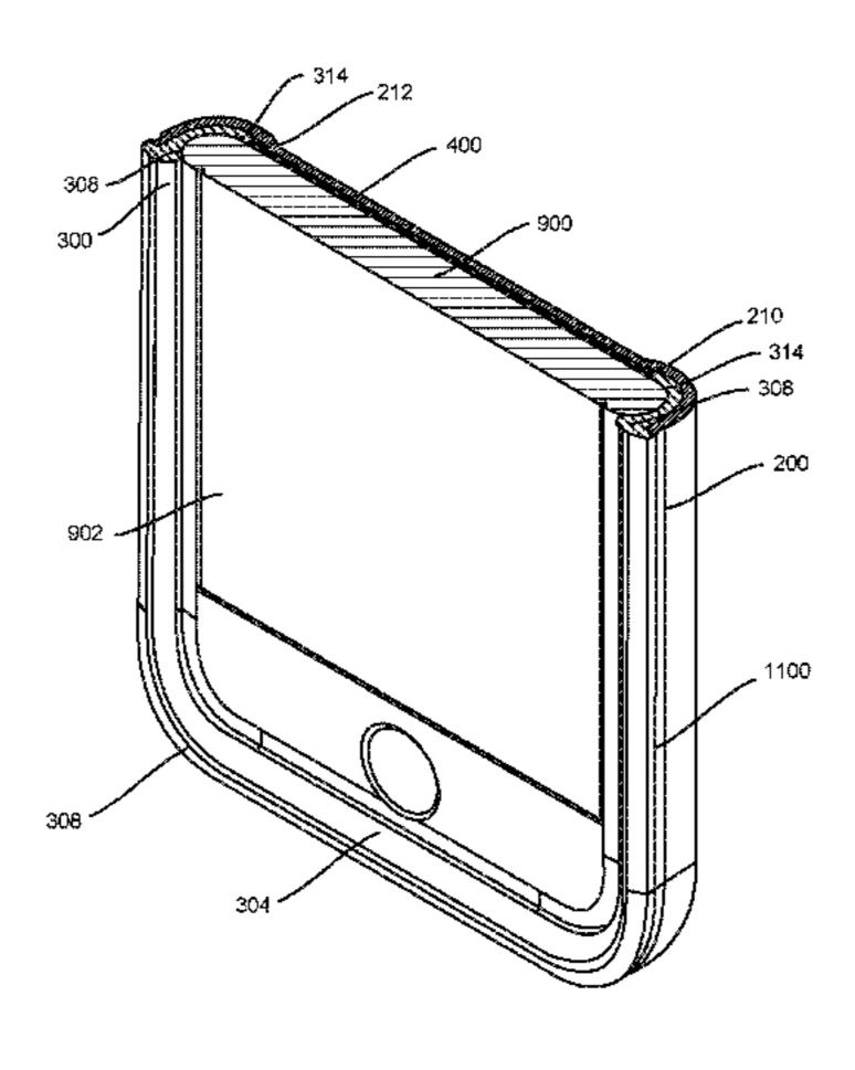
the structural member to the back surface of the installed electronic device and is at least partially bounded by the lower edge of the cushioning member.
