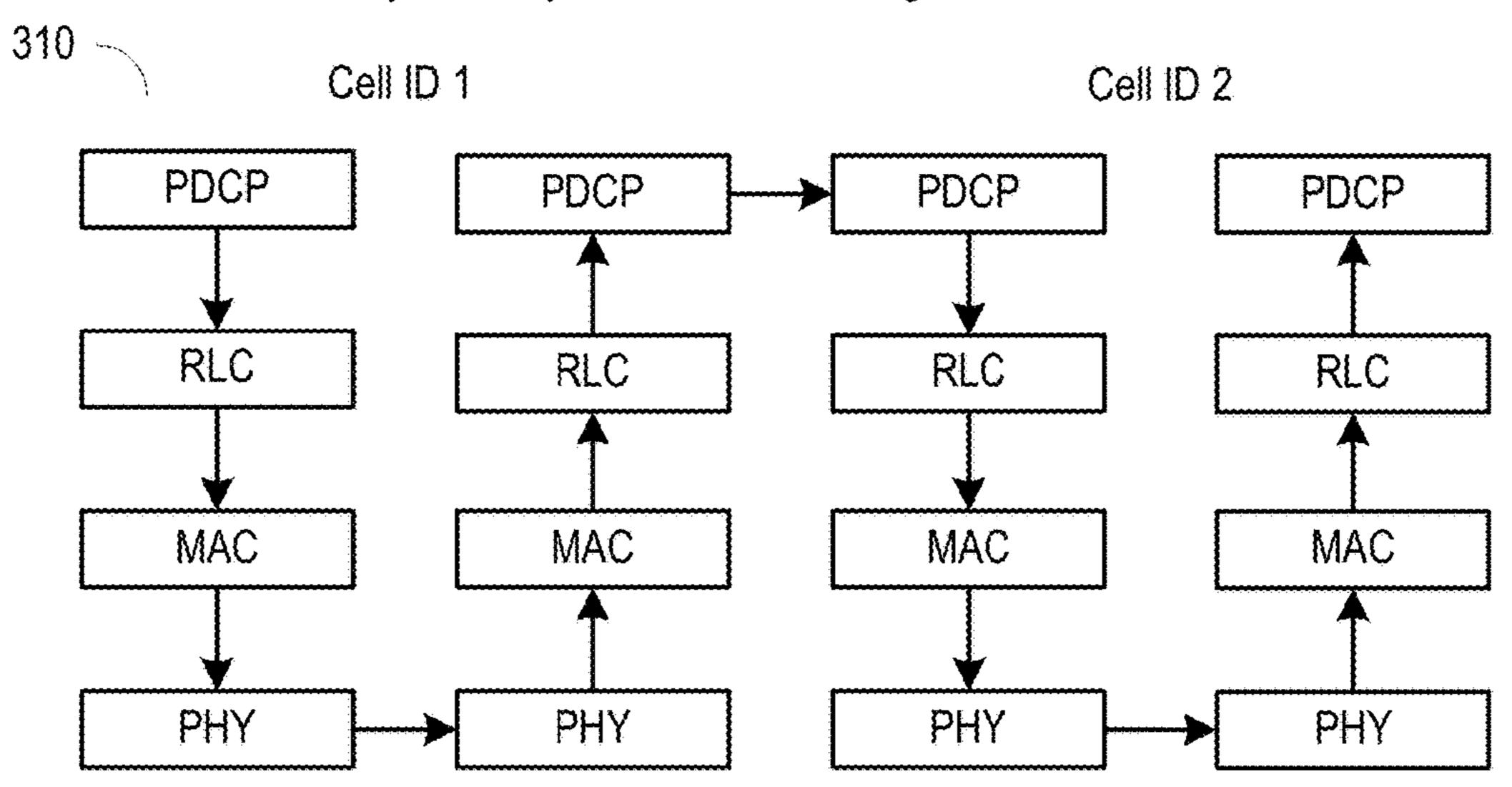
320 Layer 2 relay (switching enabled in the MAC/PHY layer)
