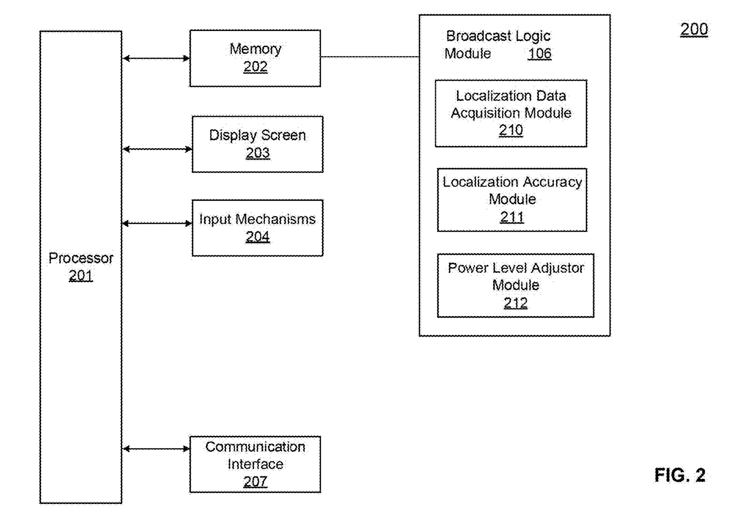
Localizing a first and at least a second mobile devices to establish respective first and at least a second estimated positions within a pedestrian area based upon fingerprint data, the mobile devices broadcasting respective localization data packets that includes the estimated positions at a first and an at least a second broadcast power levels respectively
