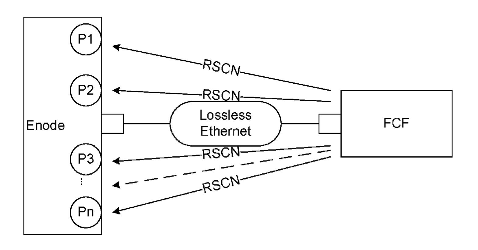
bility negotiation with the FCF, destination MAC contained in the first RSCN message being ENode MAC. Disclosed are an ENode device, an FCF and an RSCN system.
