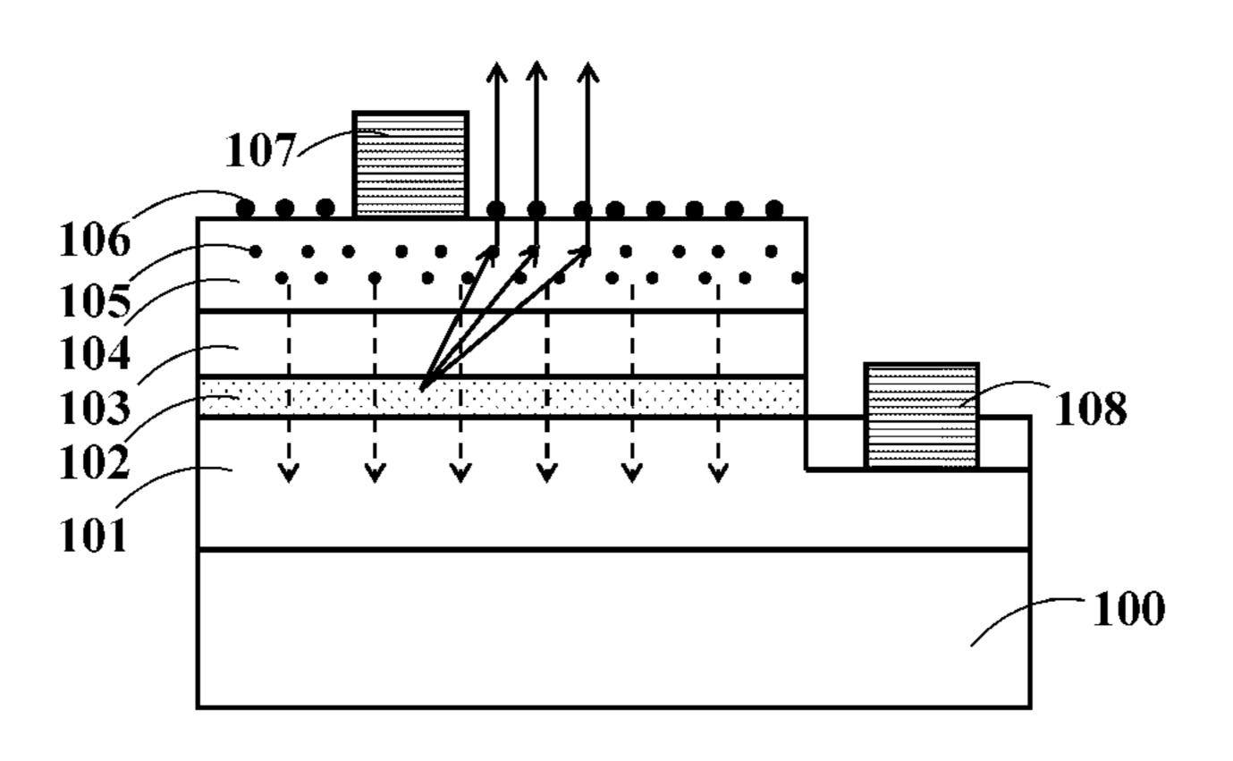
spreading layer can reduce horizontal resistance of the current spreading layer and improve horizontal spreading uniformity of current; and metal nanomaterial groups with high visible light transmittance are distributed over the upper surface of the current expansion layer for roughening and increasing light extract efficiency.
