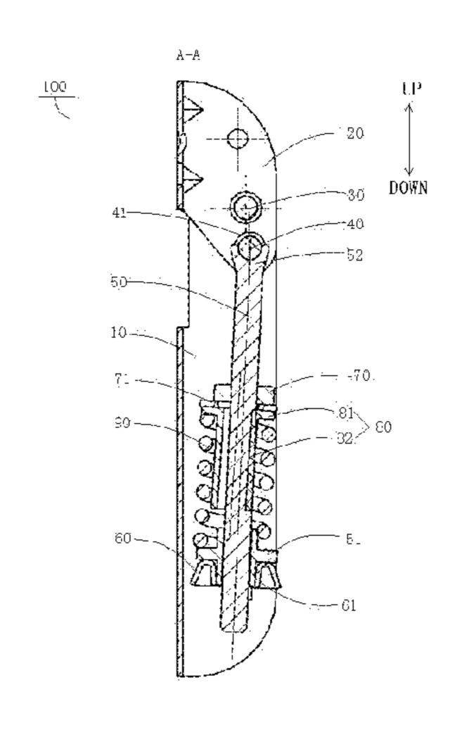
a second pivot shaft parallel to the first pivot shaft, in which both ends of the second pivot shaft may slide in the corresponding sliding grooves respectively; a guide rod; a supporting seat; a positioning part; a spring sheath fitted over the guide rod and movable between the positioning part and the supporting seat; and a spring fitted over the spring sheath.
