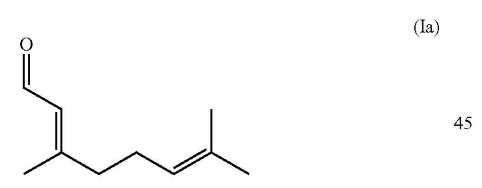
with hydrogen peroxide in the presence of a catalyst comprising a tin-containing zeolitic material of frame- 50 work structure type BEA having a tin content in the range of from 2 to 14 weight-% based on the total weight of the tin-containing molecular zeolitic material, obtaining a reaction mixture.
