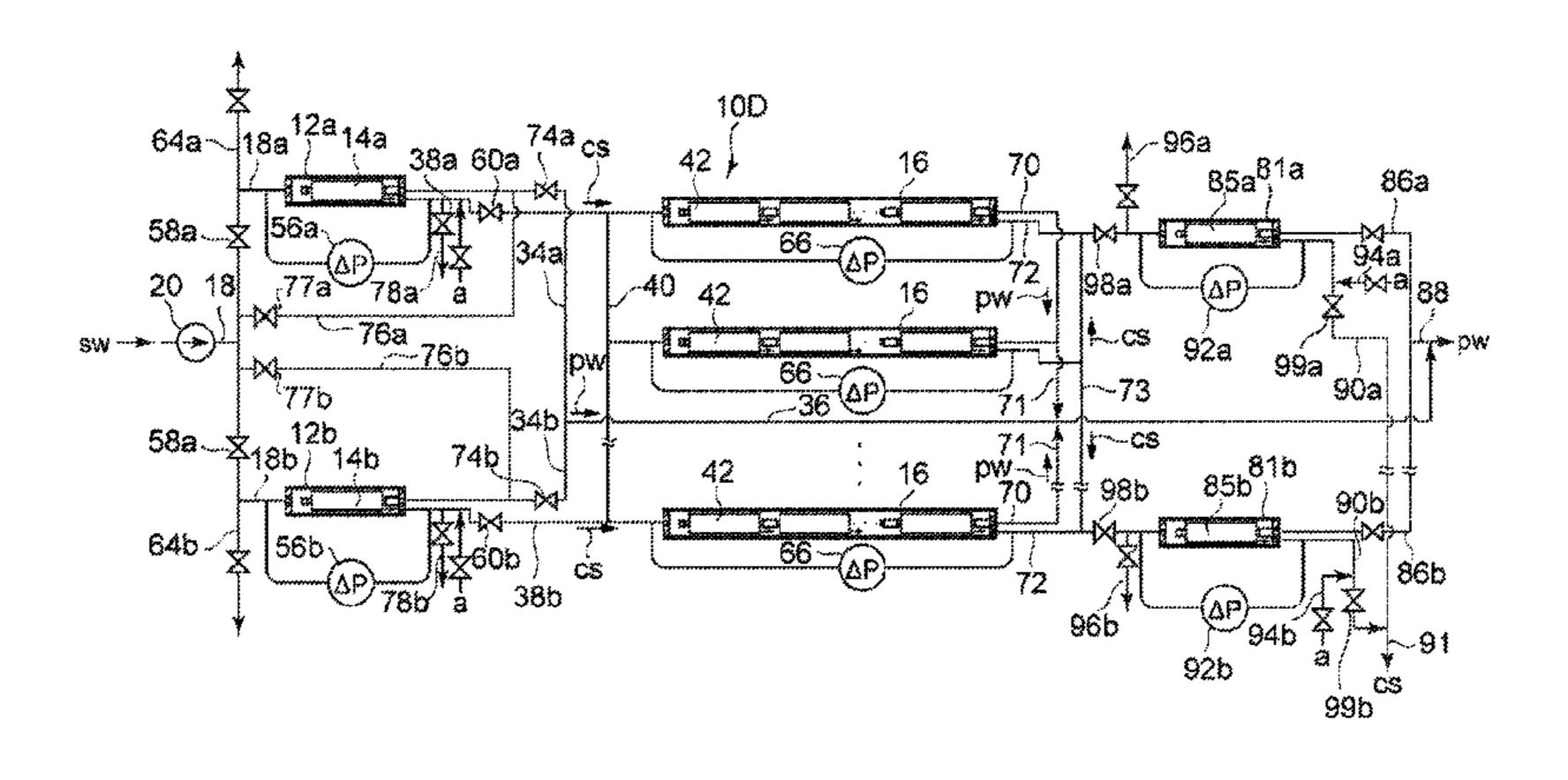
high pressure vessels 12a and 12b flows into a high pressure vessel 16. In the high pressure vessel 16, a plurality of reverse osmosis membrane elements 42 are arranged in series. When a detected value obtained by a differential pressure meter 56a or 56b provided for the high pressure vessel 12a or 12b exceeds a threshold value, introduction of the clarified seawater is stopped, and the reverse osmosis membrane element is washed or replaced.
