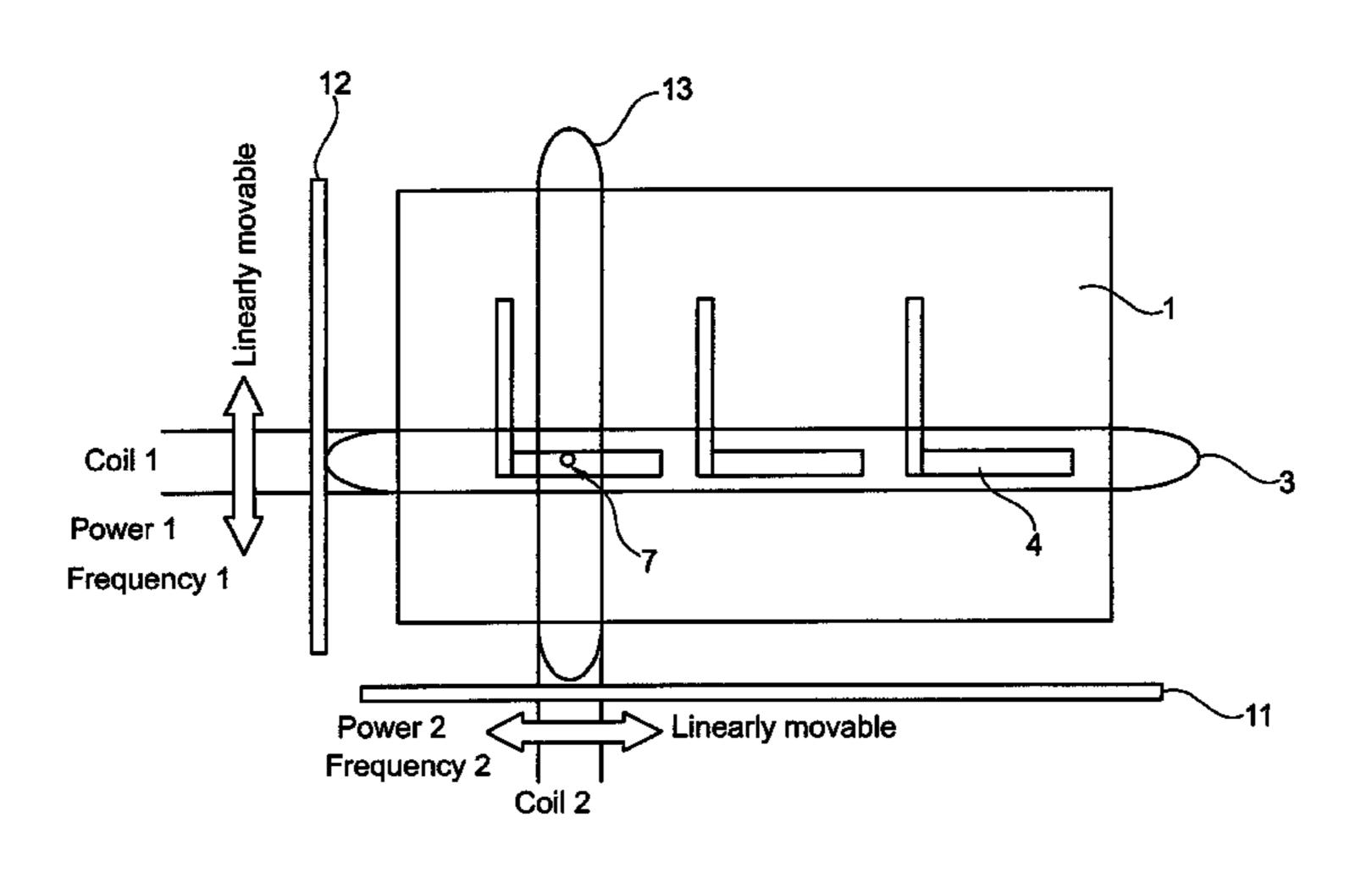
for additive manufacturing of components by selective irradiation of a powder bed, in which method the component being manufactured is inductively heated at the same time, wherein the position of one or more induction coils for inductive heating is determined and adjusted based on the geometry of the component to be produced.
