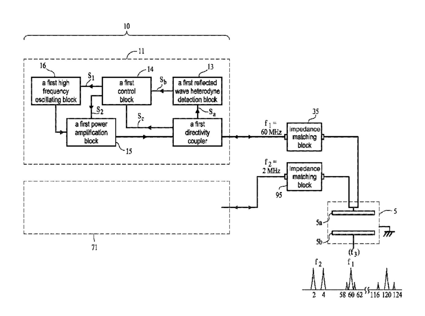
performs heterodyne detection of a reflected wave; and a first control block, which receives a signal after detection of the heterodyne detection block and a traveling wave signal, and controls an oscillating frequency of the first high frequency oscillating block and an output of the first power amplification block.
